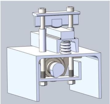
revised design which can be seen in the sketch below. It will be much lighter and could be powered by a cordless drill (or impact driver) allowing it to be independent of mains power. Weight will be greatly reduced and it will be far stiffer. A new concept of anvil
