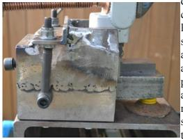
design is that changing the load on the spring with the adjusting bolt also alters the position of the anvil in relation to the striker. This in turns means
