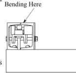
The movement on this part was severe not only upward but but at 45 degrees (see sketch). This was much more difficult to deal with as it required an increase in thickness of the material on which the striking machine
