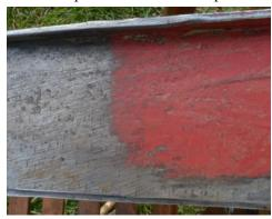
can be seen that a satisfactory result has been achieved. The thickness of the blade at the edge is approximately 0.05mm. A lick with a stone gives a usable edge.
