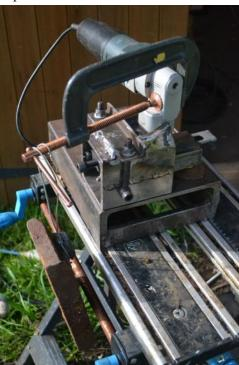
weight are an attempt to reduce further flexure of the striker mounting. In conclusion the jig works but it has some disadvantages. The first is it's weight I'm not so young any more it's true but all up it weighs at lease 20 kilos (44lb) so I wouldn't want to be carrying it around the Green Scythe Fair!! It
